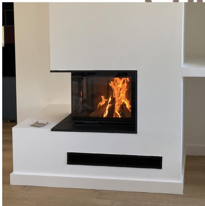
Steel insert with right serigraphic glass. Small depth of the appliance. Lift up door for wood loading. Interior made in anthracite refractory bricks. Direct connection to outside air. Glass protect system (to keep the glass clean, longer).
